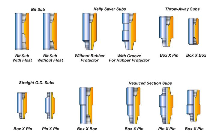
The Mechanical Properties Of All New Steel Drill Stem Subs Shall Conform To The Same Standards As DRILL COLLARS.
