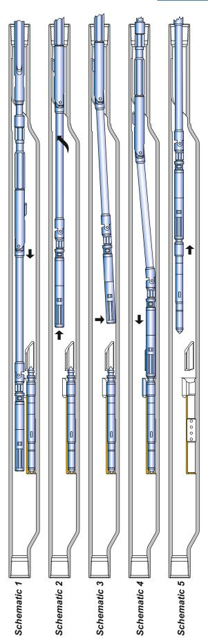
Wireline Positioning Tools are designed to provide selective location of the mandrel when there are two or more mandrels installed in a well. The tool orients in the proper position, and offsets the valve (or pulling tool) into position over the pocket for setting or retrieving.
