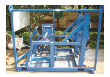
Operation of the spooler is done by hydraulic source from open-loop hydraulic power pack.
